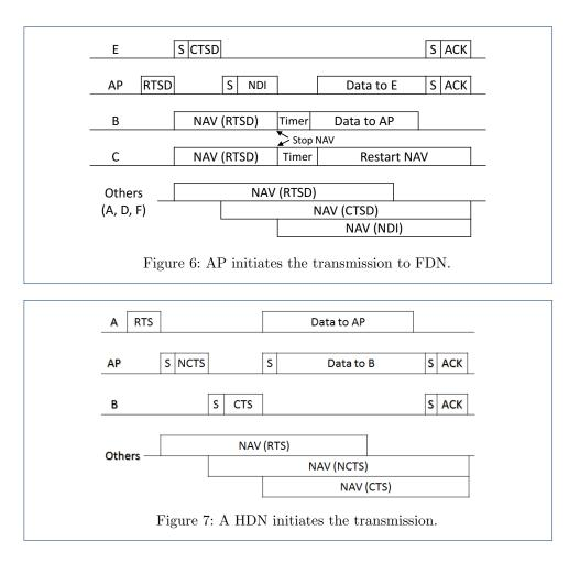
corresponding FDN also sends a CTSD with a DI value of 11 because the FDN has data for AP. BFD transmission then occurs.
