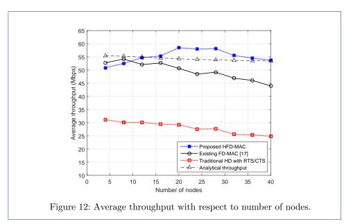
paper. The average HT ratio in practical radio environment can vary depending on various parameters, such as network topology, line of sight, transmitting power or range, etc. Therefore, we chose the average HT ratio as 30% for this simulation in Fig. 12.
